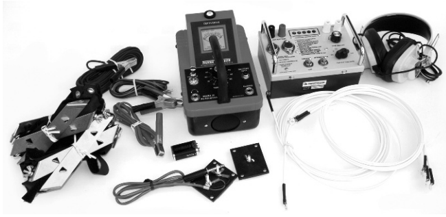
9.5 Basic equipment used for the Pearson survey. (Source: courtesy of http://www.tinker-rasor.com .)
