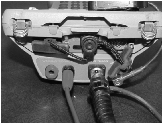
8.4 Connection of the reference electrode to the black terminal of a CIS data-logger.
