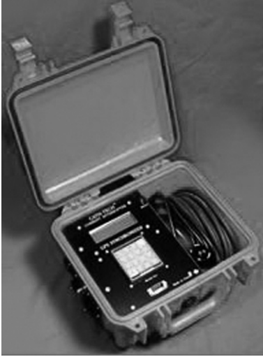
8.7 GPS synchronized current interrupter.
