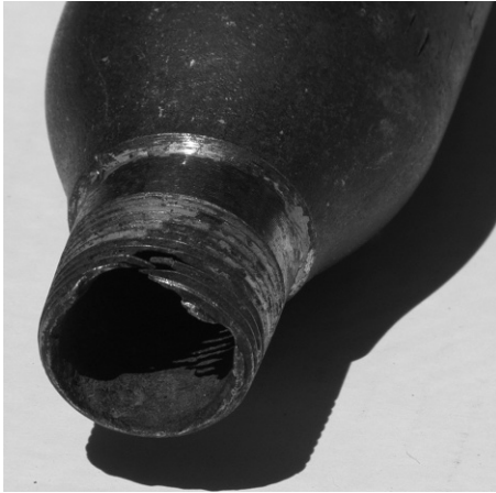
1.8 Galvanic corrosion – internal corrosion caused from using a brass valve and steel reducer in a salt water disposal system in east Texas. This reducer had to be changed every 2–3 weeks!
